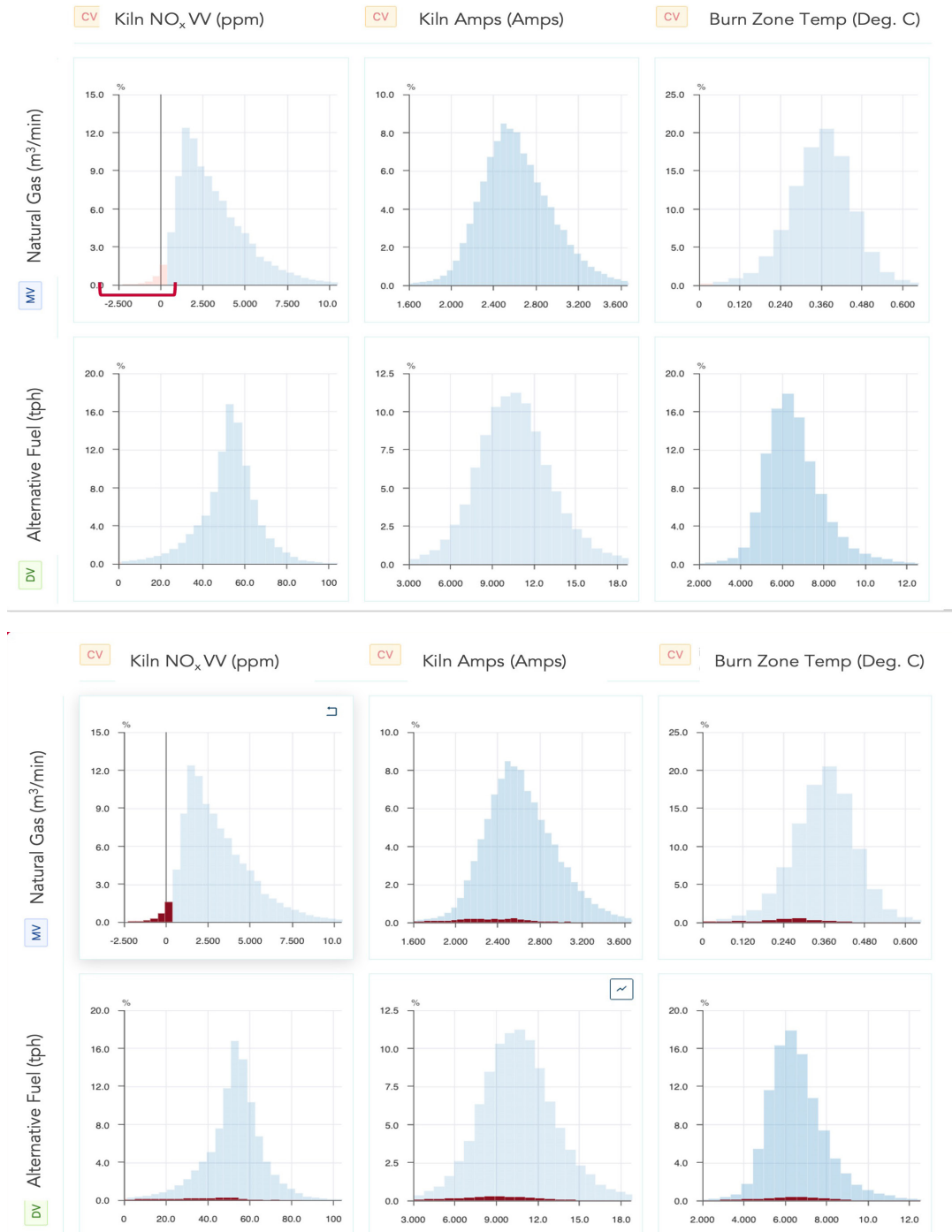
Figure 1. Unfiltered relationship matrix (top, grey) shows all possible values of each relationship learned by the AI model during training. Filtered relationship matrix (bottom, red) highlights the nonlinear relationship between natural gas flow and kiln NO x calling out behaviour of other variable pairs when this relationship is negative.
